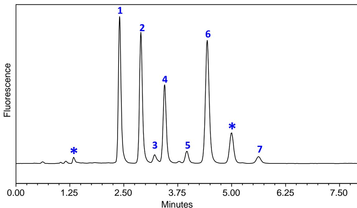
**Figure 1: DMB Labelled Sialic Acid Reference Panel Run on the LudgerSep™ uR2 UHPLC column.**
