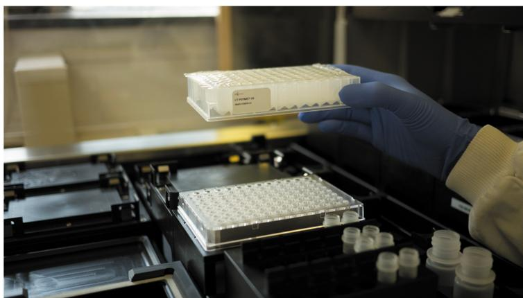
**Fig 1: HT Glycan Permethylation Microplate for mAb glycan analysis by MS**
