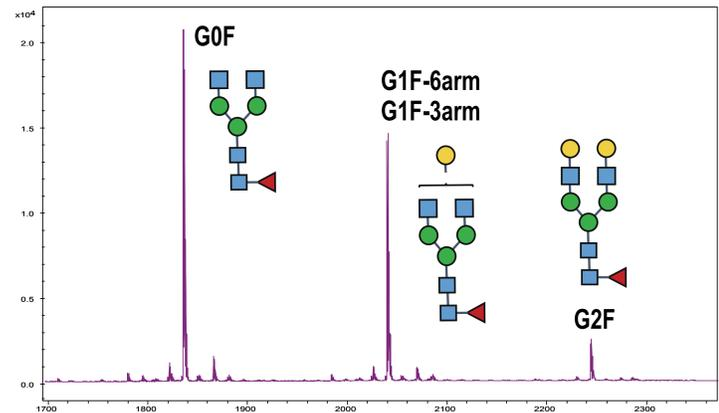
**Fig 3: Typical MALDI-MS profile of LT-PERMET-96 permethylated mAb glycans**
